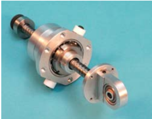
A ballscrew inerter (flywheel removed) made at Cambridge University, Department of Engineering, in 2003, designed by N.E. Houghton
