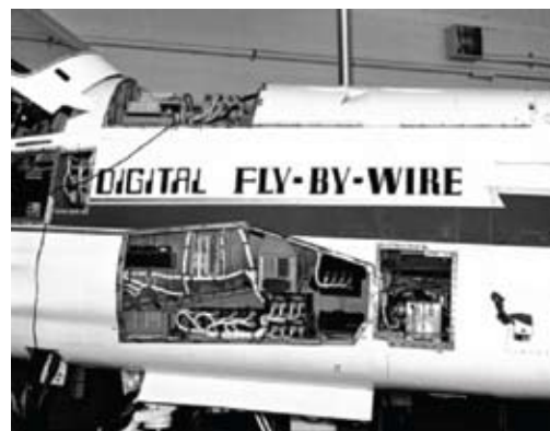
NASA used an F-8C for its digital fly-by-wire program, the first DFBW aircraft to operate without a mechanical backup system. This photo shows the Apollo hardware jammed into the F-8C. The computer is partially visible in the avionics bay. Source: NASA
