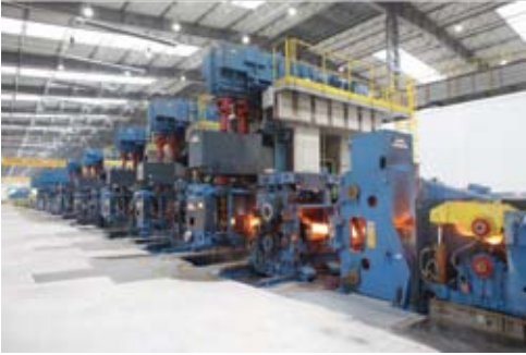
A rolling mill made of a sequence of rolling stands yielding the desired final steel bar section as the bar moves through the mill
