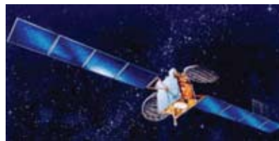
Figure 1: Structural flexible modes (above) of Astrium communication satellite platform Eurostar 2000+ (left). The shifting of frequency modes corresponds to different angular positions of the solar arrays. Source: EADS
