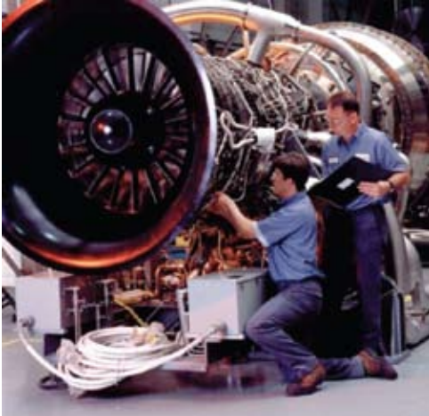
Pratt & Whitney FT8 gas turbine
