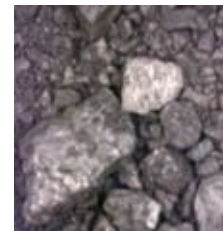
Figure 1: An image from a computer vision system on a coal conveyor is automatically processed to estimate the proportion of fines in the coal.
