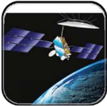
Artist's rendering of Eutelsat W2A satellite in orbit, based on the Spacebus 4000 C4 platform, with deployed solar arrays and 12-m-diameter antenna.
