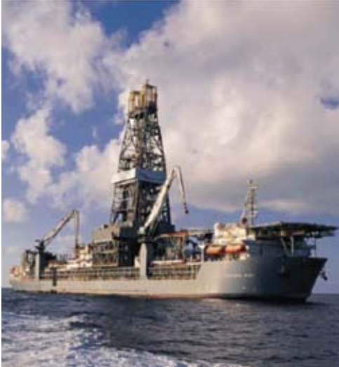
The double-hulled dynamically positioned drillship DISCOVERY SPIRIT equipped with six aquamaster thrusters
