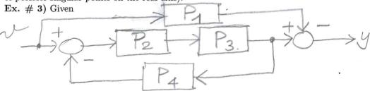
where  $\mathbf{P}_1(s) = \frac{1}{s+10}$ ,  $\mathbf{P}_2(s) = \frac{s-1}{s+2}$ ,  $\mathbf{P}_3(s) = \frac{1}{s-1}$  and  $\mathbf{P}_4(s) = -\frac{8}{s+9}$ , calculate the transfer function from v to y, the output response and the steady state output response to a constant input v. Study the observability/controllability properties of the series  $\mathbf{P}_2(s)$  with  $\mathbf{P}_3(s)$ .
