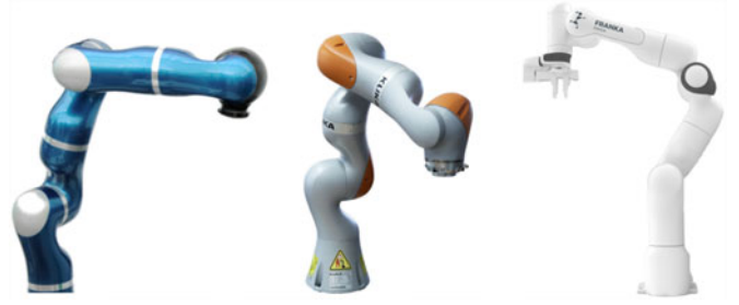
Fig. 2. From left: the DLR LWR-III (by courtesy of DLR), the KUKA LBR iiwa, and FRANKA EMIKA (by courtesy of FRANKA EMIKA GmbH).
