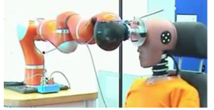
Fig. 11. Collision experiment (DLR/KUKA LWR and Hybrid III dummy).
