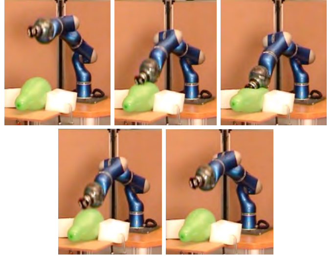
Fig. 2. Collision with a balloon (motion at 100^\circ/\text{s} ) and robot reaction
