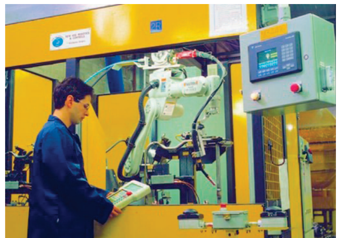
Fig. 9. Lead-through programming by teach pendant.
