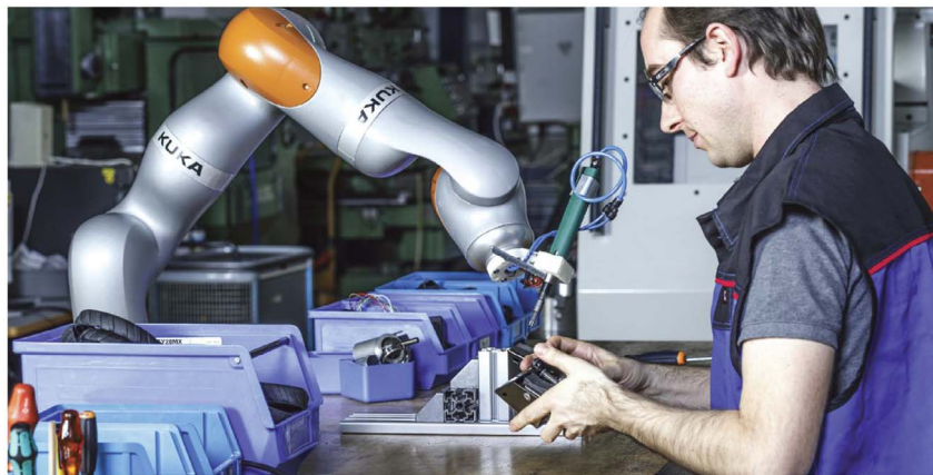
(b) Collaborative robot allowing the human worker to stand in its proximity and work together at the same task.
