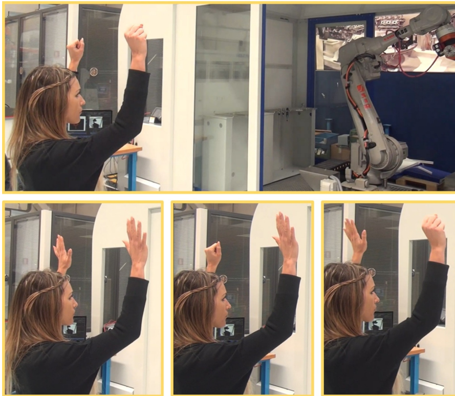
Fig. 23. Examples of gestures being performed by a user to command the robot.
