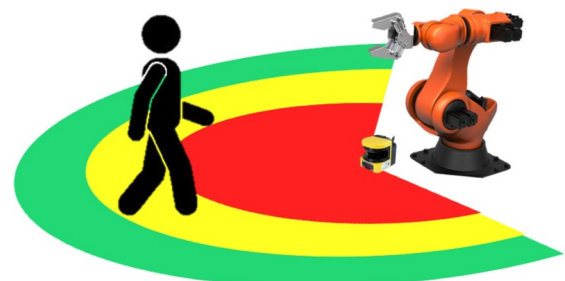
Fig. 2. Safety zones for human–robot collaboration with speed and separation monitoring technology (Courtesy of ABB Robotics).
