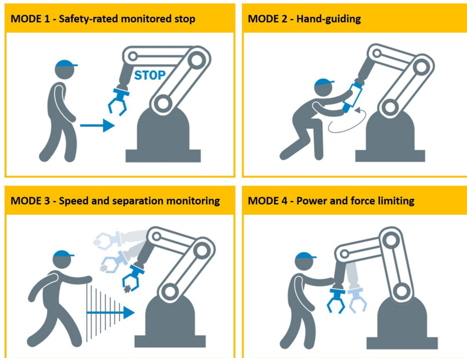
Fig. 1. The four forms of collaboration identified by the robot safety standards ISO 10218-1/2 [22,23] and by the technical specification ISO/TS 15066 [24].
