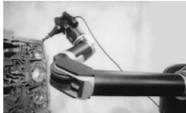
WAM cable-driven robot (Whole Arm Manipulation) by Barrett Technology [Salisbury, 1988]
