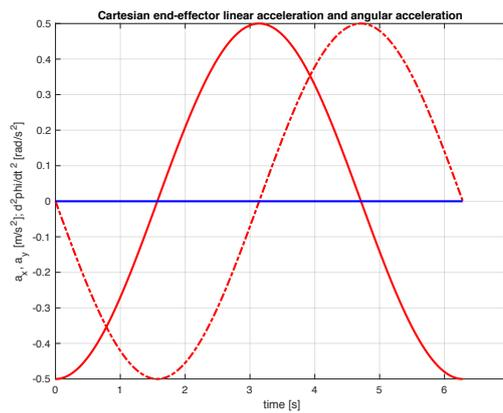
Figure 6: Cartesian linear acceleration  $\ddot{\mathbf{p}}(t)$  ( $a_x(t)$  [red],  $a_y(t)$  [red, dashed]) and angular acceleration  $\ddot{\phi}(t)$  [blue].
