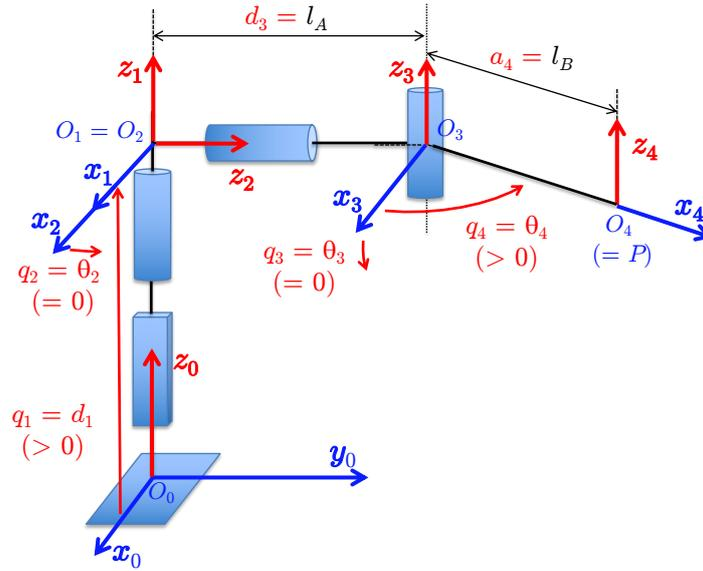
Figure 3: Assignment of DH frames for a PRRR robot.
