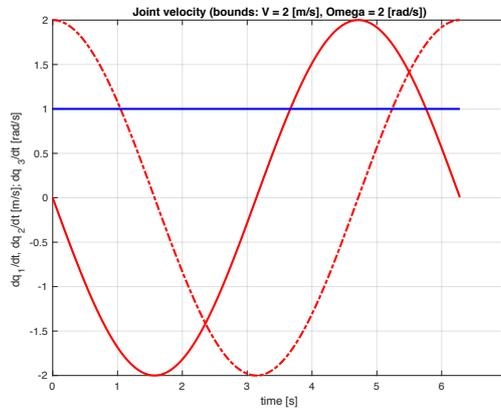
Figure 8: Joint velocity  $\dot{\mathbf{q}}(t)$ :  $\dot{q}_1(t)$  [red],  $\dot{q}_2(t)$  [red, dashed],  $\dot{q}_3(t)$  [blue].
