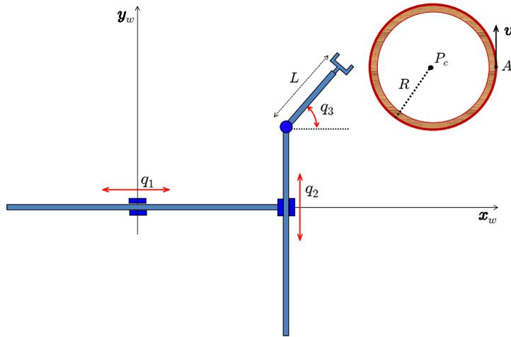
Figure 2: The planar PPR robot and the Cartesian task to be executed.
