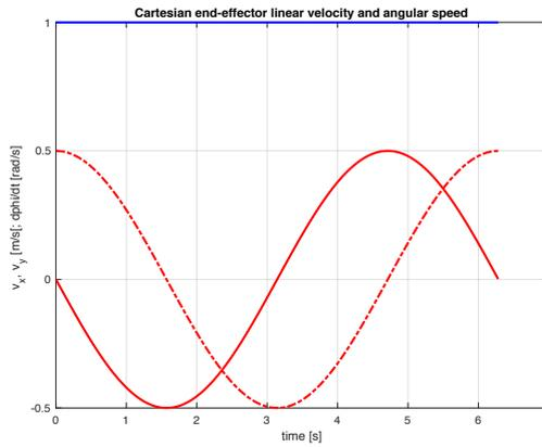
Figure 5: Cartesian linear velocity  $\dot{\mathbf{p}}(t)$  ( $v_x(t)$  [red],  $v_y(t)$  [red, dashed]) and angular speed  $\dot{\phi}(t)$  [blue].
