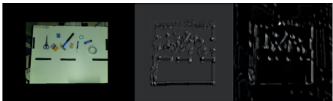
Figure 3: From left to right: Input image of a set of real objects, the visual features extracted from the CNN of a YOLO network, and the associated Grasping Features. The GFs have intensity peaks at the image points of possible grasp positions, while visual features recover just object shapes.
