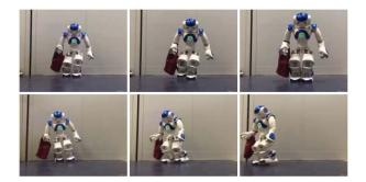
Fig. 2. NAO walks carrying a swinging bag: robust IS-MPC (top), nominal IS-MPC (bottom). With robust IS-MPC, compensation of the midrange disturbance produces a slight leaning action against the disturbance, while ZMP constraint restriction provides robustness to the time-varying components of *w*. On the contrary, nominal IS-MPC struggles to maintain balance and visibly deviates from a straight line path.
