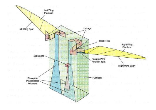
Robofly is actuated by a pair of piezoelectric actuators, that control the angle of the wing support with respect to the body. The angle of attach is a function of the rotation speed of the wing support.
