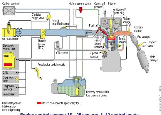
Engine control system: 15 – 25 sensors, 8 -12 control inputs,
