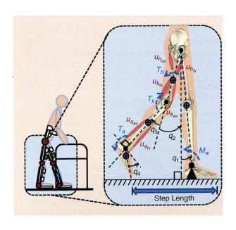
A four-link gait model based on a subject wearing a hybrid neuroprosthesis and using a walker for trunk stabilization.
