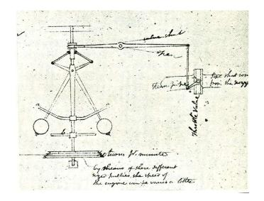
In 1789, Boulton & Watt, used same principle to adjust the steam inlet valve of a steam engine.
