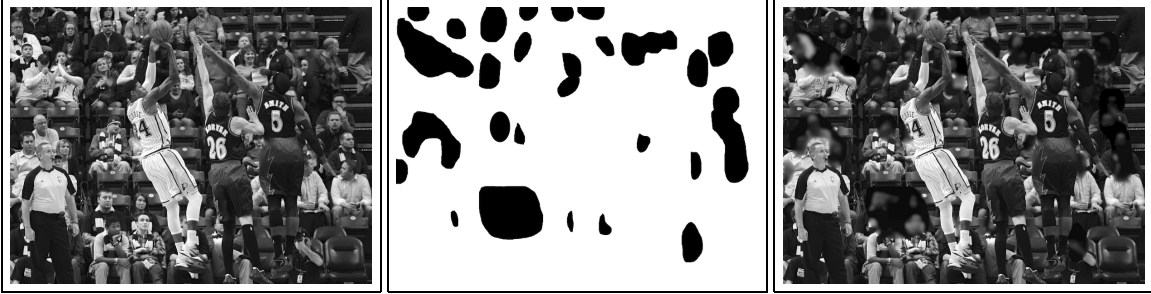
Figure 5: Masked blur filter example: original 3114 \times 2376 image (left), filter mask (center), filtered image (right).
