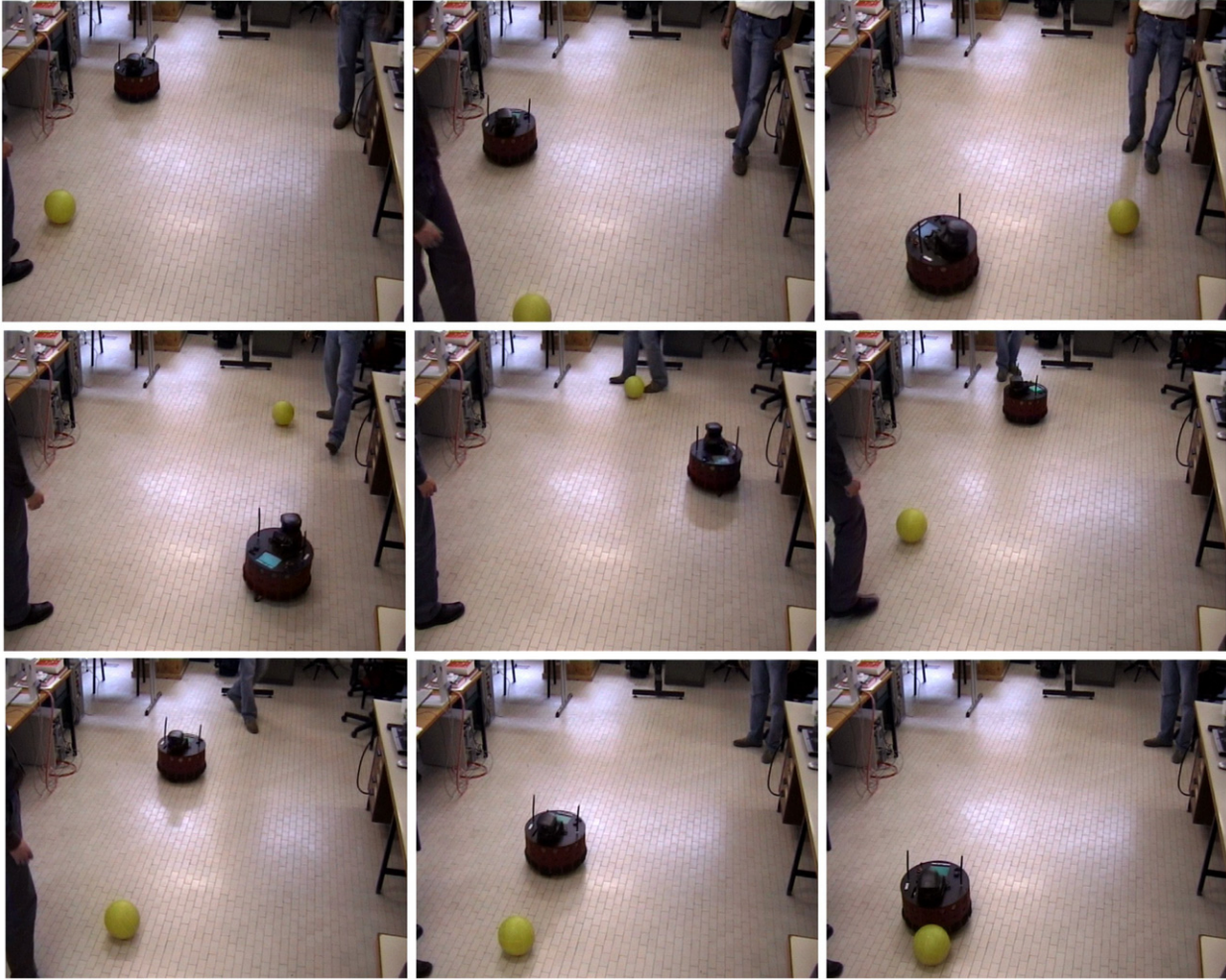
Fig. 16. An experiment where the robot tracks and intercepts a ball passed back and forth by two human players.
