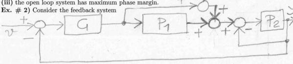
with  $\mathbf{P}_1(s) = \frac{1}{s(s+2)}$  and  $\mathbf{P}_2(s) = \frac{s-2}{s^2+s+3}$ . Design a controller  $\mathbf{G}(s)$ , with dimension  $\leq 2$ , such that the closed-loop system is asymptotically stable with
