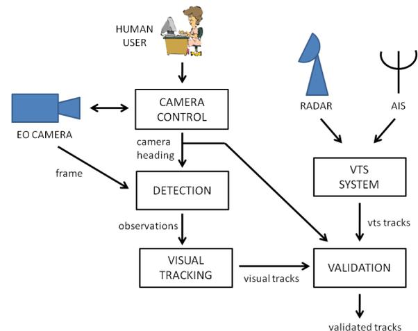
Figure 1: Architecture of a VTS/Coastal Surveillance Site
