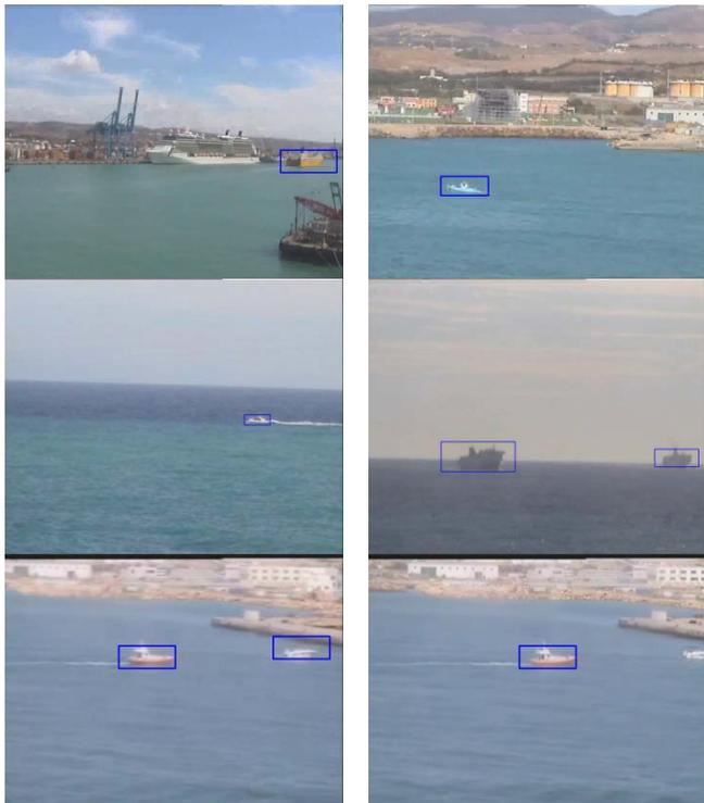
Figure 3. Boat detection using the proposed method on different videos from the MarDCT data base. The algorithm runs at multiple scales and can detect vessels of different size with varying lighting conditions.
