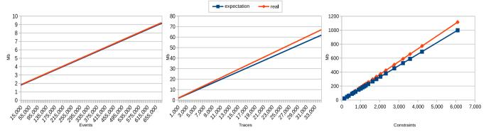
Fig. 4. The space consumption is linearly dependent on the total number of events in the log (left), number of traces in the log (center), and number of rules to check (right).
