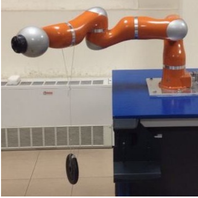
Fig. 6. A known mass hanging at a known point of link 4 of the KUKA LWR mimics the point-wise application of a pure force in static conditions, and is used for validating the proposed contact force estimation method
