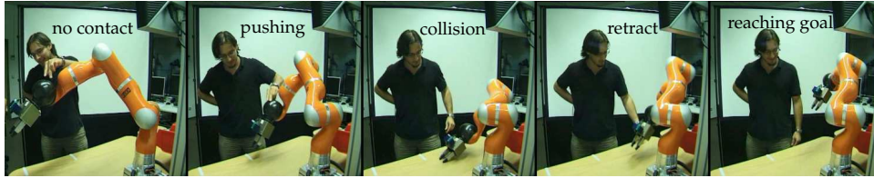
Figure 6.22: The robot is pushed by the human and thus deviates its trajectory. Since the robot has no knowledge about the position of the table, the robot collides into the table. However, it smoothly and quickly recovers from this rigid contact due to the deformation of the path and the used impedance control. Finally it reaches the desired goal configuration x_d^* . The external forces are obtained with the nonlinear observer based on the generalized momentum.
