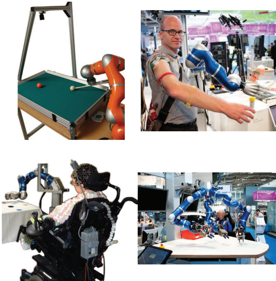
Figure 11.1: Several example setups using the developed safety oriented state based robot control architecture. LWR-III controlled via Brain-Machine Interface, SAPHARI setup, Billiard playing and EMG-controlled robot.
