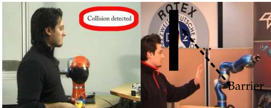
Figure 3.20: Real collisions with the chest and arm were conducted up to a robot velocity of 2.7 m/s.
