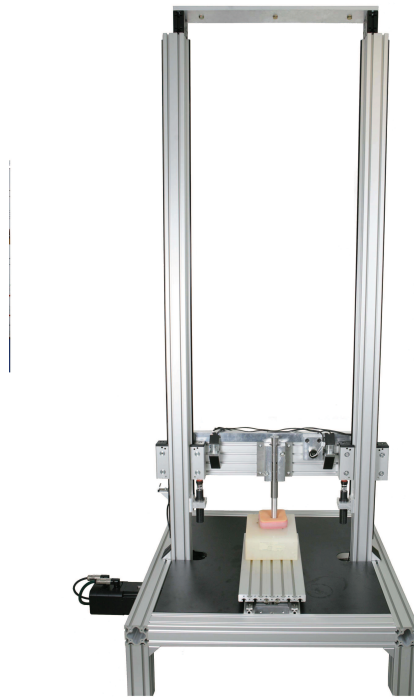
Figure 10.6: Drop testing setup for analyzing soft-tissue injury during blunt and sharp contact.
