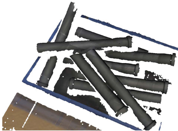
Figure 7.10: Generated 3D model from a series of sweep scans over the filled bin.
