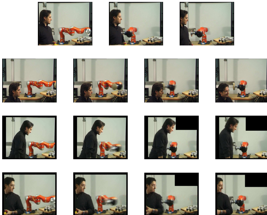
Figure 4.13: Impact tests with a human chest at 2.7 m/s and head at 1.5 m/s. The impact velocities for the abdomen and the shoulder were as well 2.7 m/s which is the maximum velocity of the robot. During all these experiments the robot does not react to the activated collision detection. During all these tests the robot stopped only due to an exceedance of the maximum nominal joint torques. However, as a result from the crash test dummy experiments, the impact forces caused by the very short collision duration cannot be affected by this feature due to its delayed reaction. These test were initially shown in [92] and support if not even prove the previously given conclusions.
