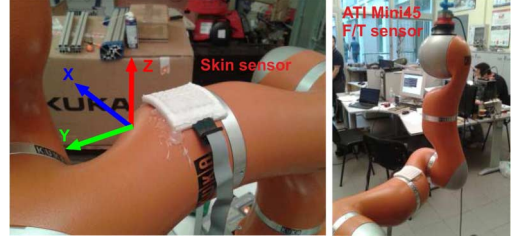
Fig. 8. The skin sensor installed on the 3rd link of the KUKA LWR4.
