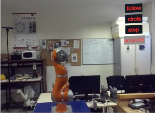
Fig. 4. The mixed reality user interface on the Rift HMD screen lenses.
