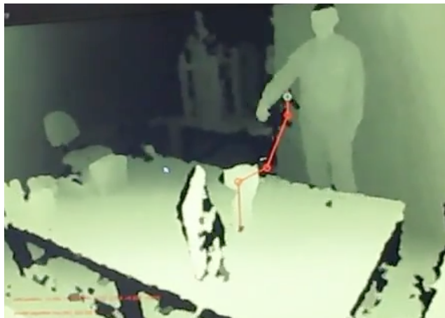
depth image and human-robot distance computation
