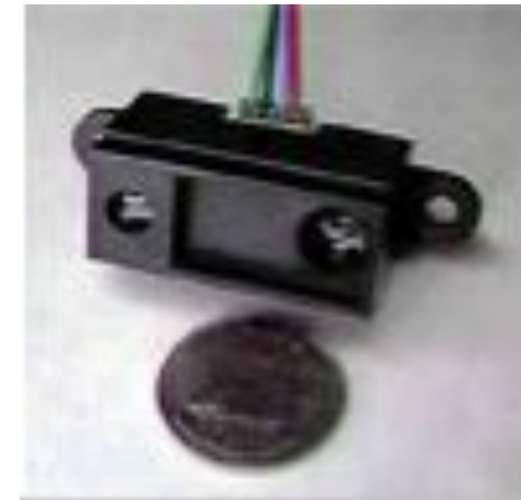
IR sensor SHARP GP2 (supply 5V, range 10 \div 80 cm)
