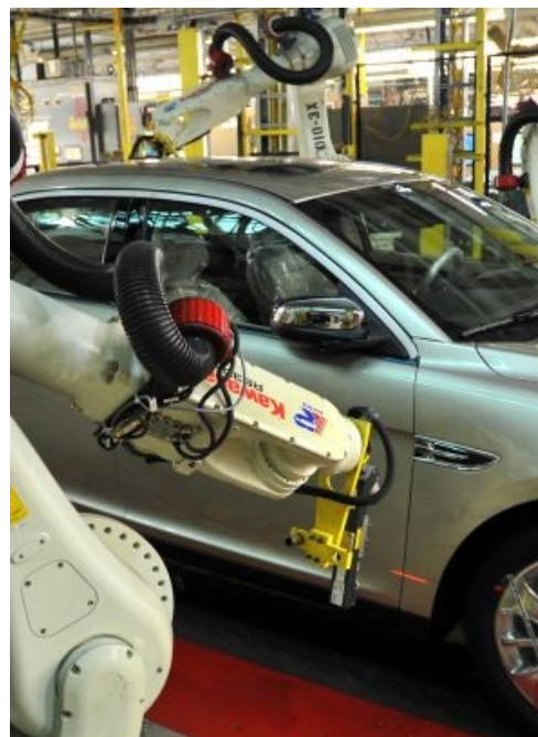
Structured light approach to best fit and finish car bodies (down to 0.1 mm) for reducing wind noise [Ford Motor Co.]
