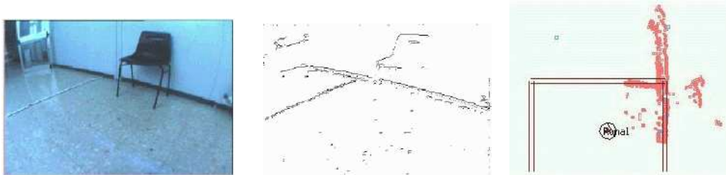
Fig. 6. Vision based range data extraction (office environment)
