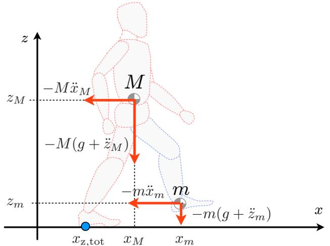
Fig. 1. 2-mass model in the sagittal plane.
