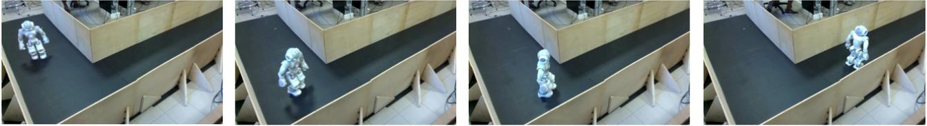
Fig. 10. Second experiment: negotiating a turn. In the first snapshot NAO is approaching a left turn. The subsequent snapshots show how the robot correctly detects the corner and keeps the center of the corridor also during the turn.
