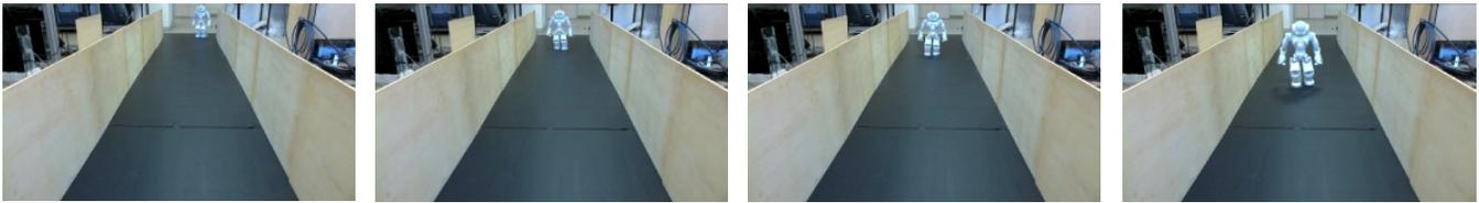
Fig. 9. First experiment: vision-based corridor navigation with off-centered start. The first two snapshots show NAO starting away from the corridor center but rapidly recovering it. The last two snapshots illustrate how NAO is able to keep walking at the center of the corridor.
