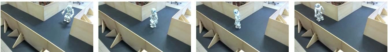
Fig. 11. Third experiment: turning at a T-junction. The first snapshot shows NAO approaching the junction. When the junction is detected the robot takes the specified direction (second and third snapshot) and resumes walking at the center of the corridor (fourth snapshot).
