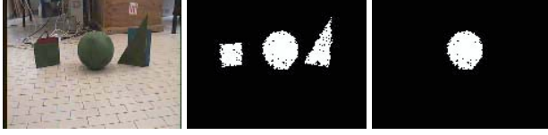
Fig. 4. Left : Three objects with the same color. Center : After color recognition and filtering. Right : After shape recognition.
