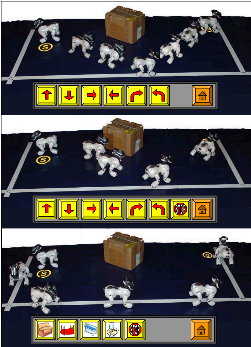
Fig. 3. Comparing navigation modes: AIBO is driven from S to G with single step (above), semi-autonomous (center) and autonomous (below) modes. The ASPICE Navigation GUIs for each mode are also shown; in each GUI, the home button brings back to the ASPICE main GUI.
