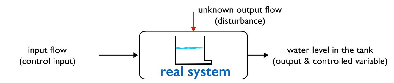
problem: we want to maintain the water level at a desired height regardless of the unknown output flow and any other disturbance
