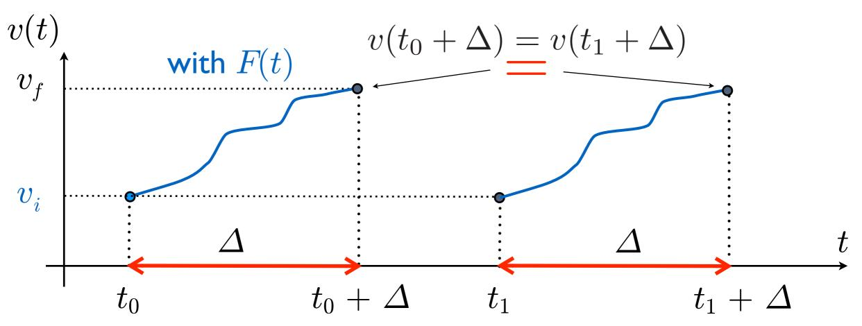
same initial condition  $v_i$  and same input (force) F(t) after same time interval  $\Delta$  leads to the same state
