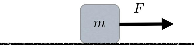
$$\begin{array}{ll} {\rm model} & \dot{v} & = & \displaystyle \frac{F}{m} \\ {\rm (linear differential equation)} & v(0) & = & v_0 \end{array}$$
