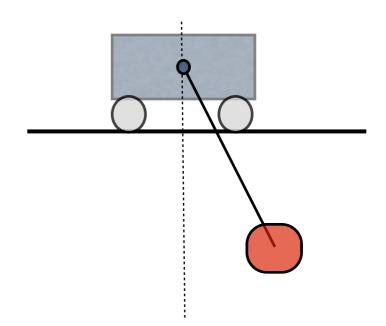
crane control: input shaping technique (Georgia Tech)
