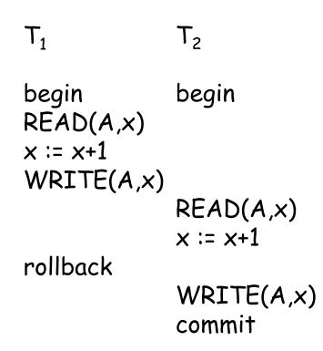
The problem is that T2 reads a value written by T1 before T1 commits or rollbacks. Therefore, T2 reads a "dirty" value, that is shown to be incorrect when the rollback of T1 is executed. The behavior of T2 depends on an incorrect input value.
