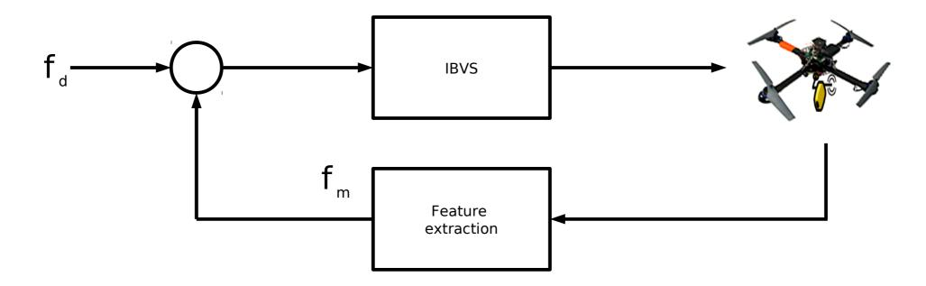
Visual error on image plane (tracking a desired target/object)
